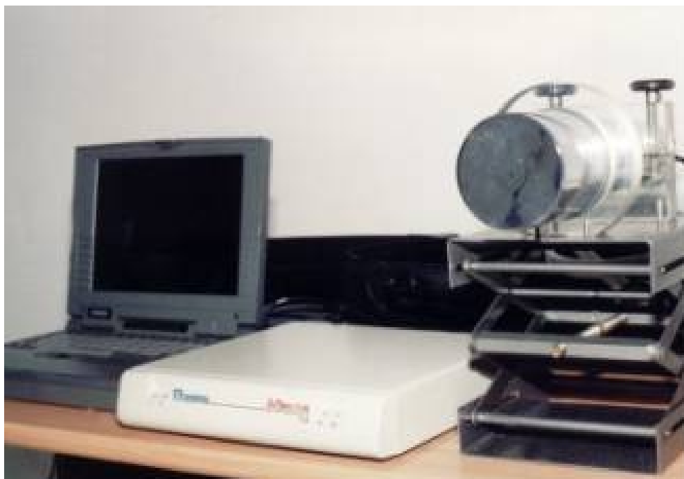
FIG.1. Mobile detection unit for I-131 and Tc-99m measurements
