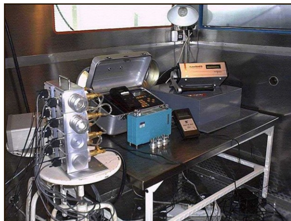
Figure 3. Radon and radon progeny monitors in the calibration chamber
